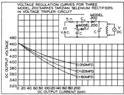
components in many television receivers. The Model 200 Rectifier is designed and engineered to meet the requirements of 7" and 10" television receivers, both in current handling capacity and temperature rise above ambient conditions. By the use of Model 200 Rectifiers in the power supply, the television manufacturer can decrease the size, cost and weight of his receiver and provide improved performance and long life.
