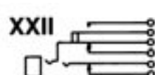
XXII Double closed circuit. Isolated switching "make" circuit on ring spring. (J7-1A).
